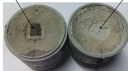
Fig. 6 Specimen autopsied across the steel mortar interface
